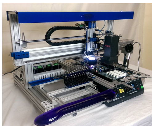
SM-300 BGA Rework Station
