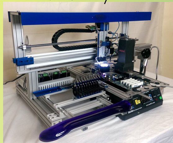
SM-300 BGA Rework Station
