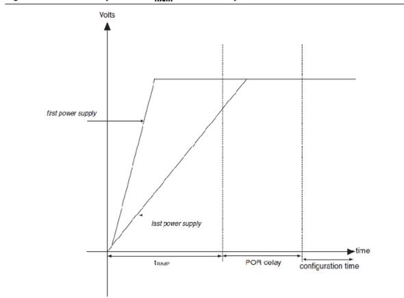
図 5.2.5.1 Relationship between  $t_{RAMP}$  and POR Delay
